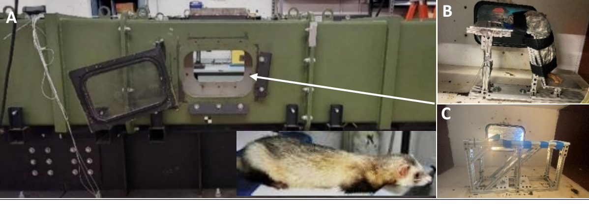
Large shock tube for ferret blast exposure. Tube has been modified to expose the ferret. (A) Arrows show the testing section of the shock tube. (B) Upright fixture. (C) Prone fixture. A stuffed animal was used for demonstration.
