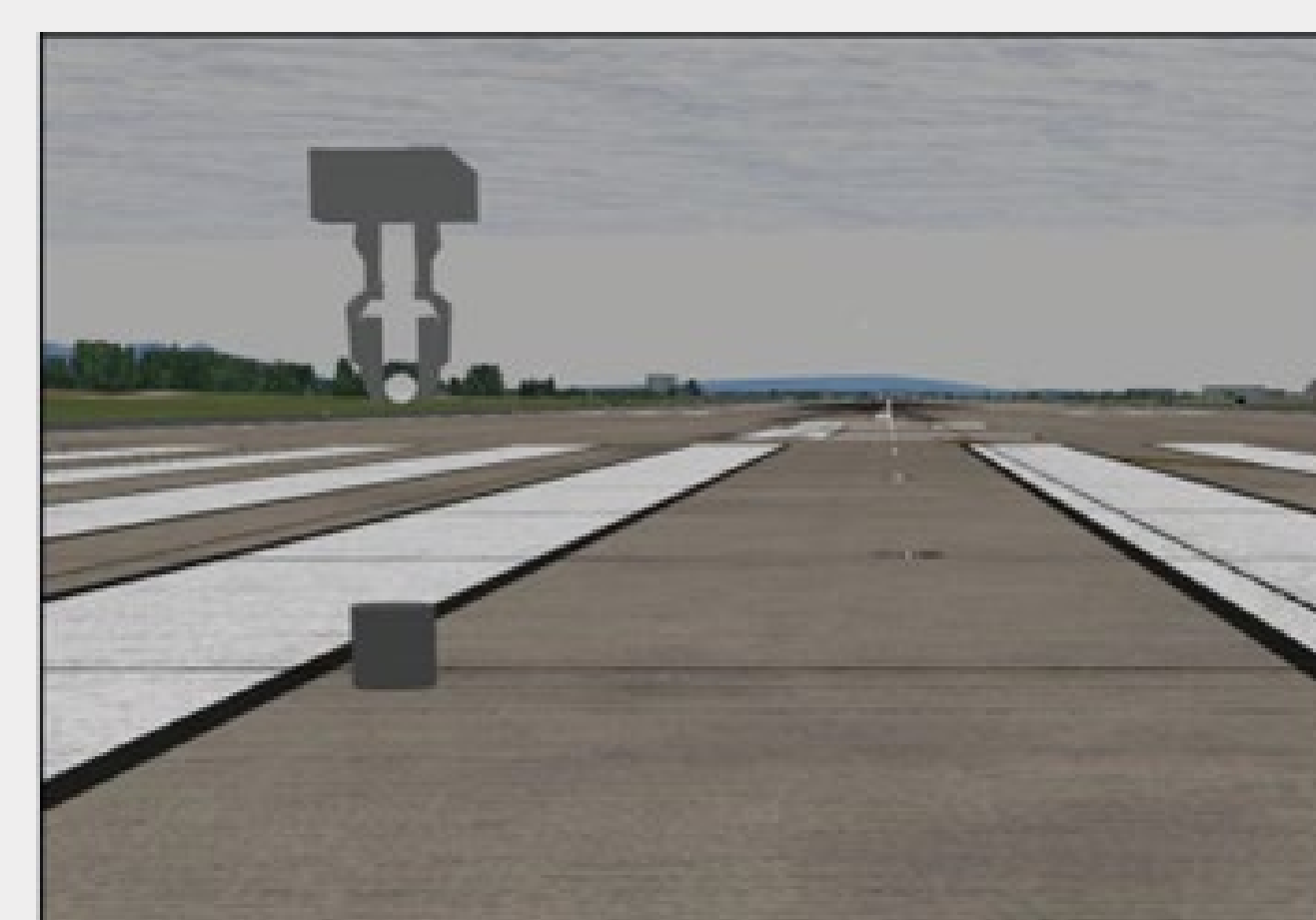
Figure 4. Gripper Task. The operator is required to perform a simulated telerobotic arm task using a 3D display. The objective is to assess operationally relevant stereoscopic remote vision system (RVS) performance in a way that can be mapped to underlying visual capabilities (photo by authors).
