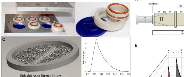
In Vitro stretch injury of cultured neurons. Study of neuronal response to high rate deformation. Allows the investigation of injury mechanisms in real time.
