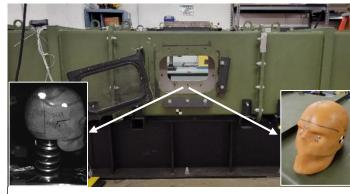
Instrumented dummy head with biofidelic neck. This head has been used in the CIBM<sup>3</sup> to determine the incident pressure acting on the head under helmeted and unhelmeted exposure to blast. Arrows show the testing section of the human scale shock tube.
