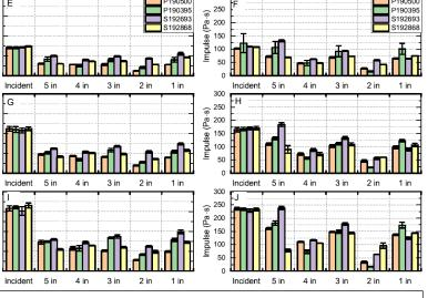
(ICP) measurements in the human head. (A-B) PHMS instrumented with intracranial pressure sensors at five locations. D) ICP traces from 70kPa BOP. (E-J) ICP peaks and impulses from 70, 130, 180 kPa BOP.
