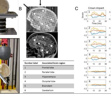
Human Scale Surrogate for Blunt Impact Testing. (A) Surrogate attached to a Hybrid III anthropomorphic neck with clear ballistic gel and markers for motion tracking. (B) Six brain regions of interest for spatial strain distribution. (C) Temporal strain histories for each region.
