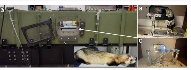
Large shock tube for ferret blast exposure. Tube has been modified to expose the ferret. A) Arrows show the testing section of the shock tube. B) Upright fixture. C) Prone fixture. A stuffed animal was used for demonstration.
